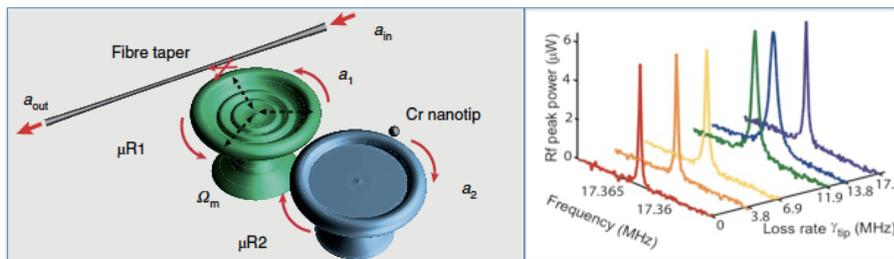
Figure 1. Left panel: a phonon laser formed by two coupled resonators. Right panel: Linewidth variation in a phonon laser tuned around an EP.
