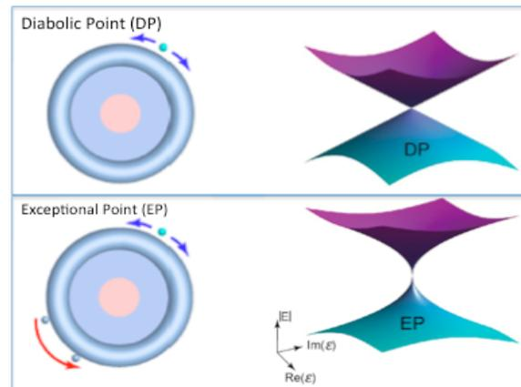
Figure 2. Upper panel: a WGM sensor operated around a diabolic point (DP). Lower panel: a WGM sensor operated around an exceptional point (EP).
