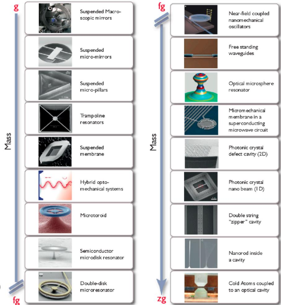
**Figure 1:** Left: canonical cavity optomechanical systems. Right: diverse range of architectures. Images from M. Aspelmeyer, T. J. Kippenberg, and F. Marquardt, *Cavity Optomechanics* arXiv:1303.0733 (2013).
